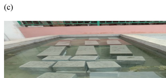
Fig. 2 a Reinforcement cages, a-1 20 mm cover cage, a-2 30 mm cover cage, a-3 40 mm cover cage b casting in wooden moulds c curing under water
